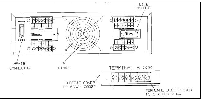
Figure 2-2. Rear Panel Detail (6624A Shown)
